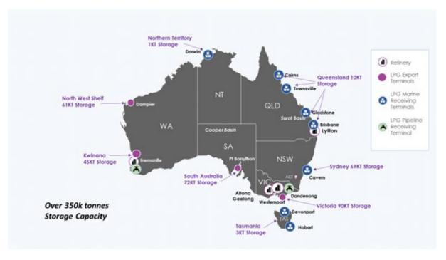
Figure 19 shows that the LPG industry has significant marine port storage capacity – over 350k tonnes.
